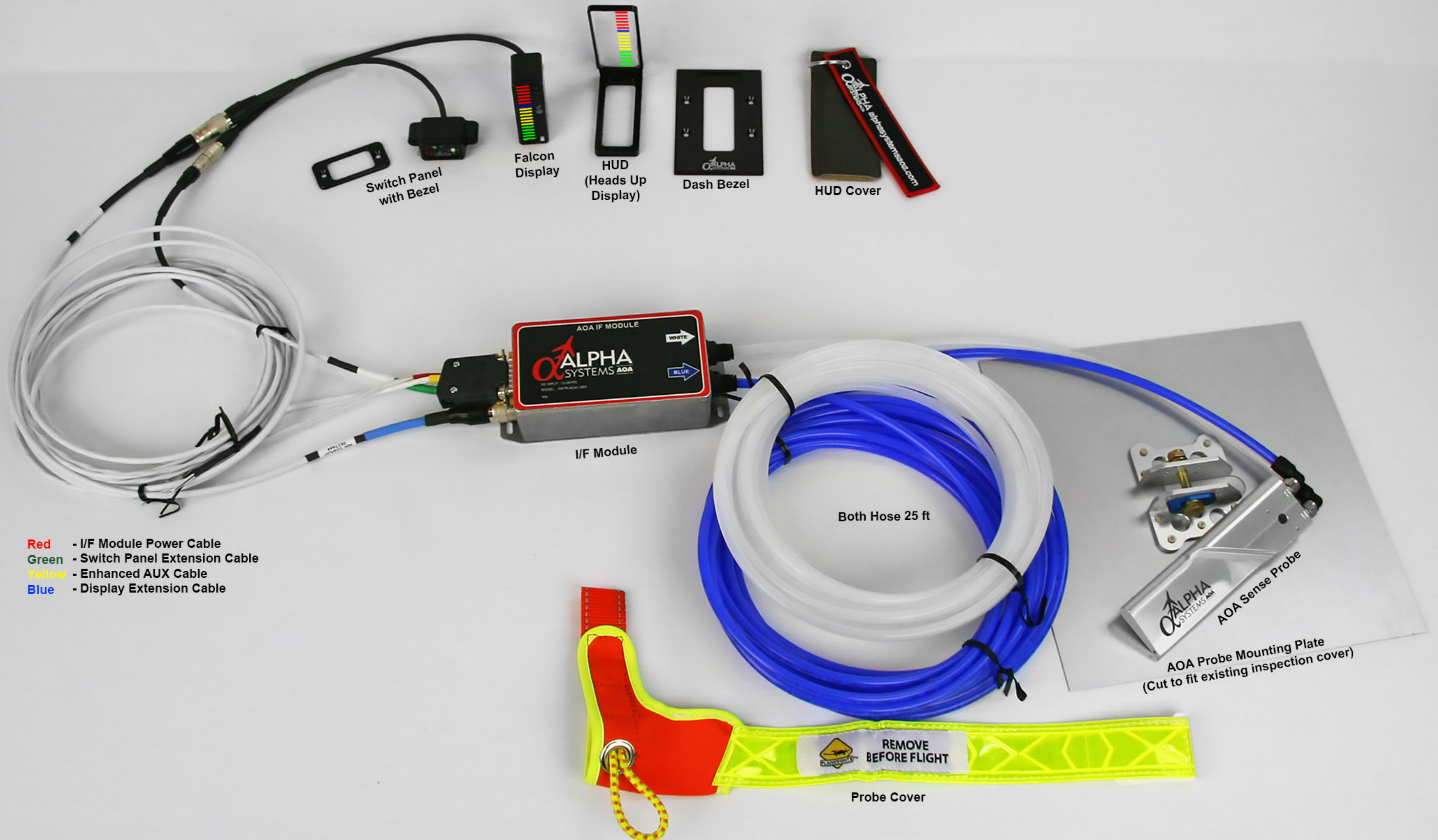
Alpha Systems AOA Falcon HUD System Diagram DSTR-AOA-9200K-(HUD)
